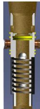
Tool can be hydraulically reset (unlocked) downhole by dropping 2 steel deactivation balls. Locking Ball and Activation Ball will Shear and FLOW to BIT resumed.
