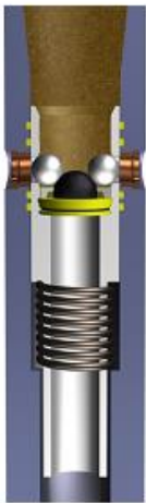
De-Activation Balls Dropped PRESSURE UP
