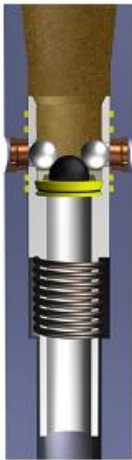
De-Activation Balls Dropped PRESSURE UP
