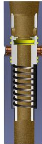
Drilling Mode FLOW to BIT
